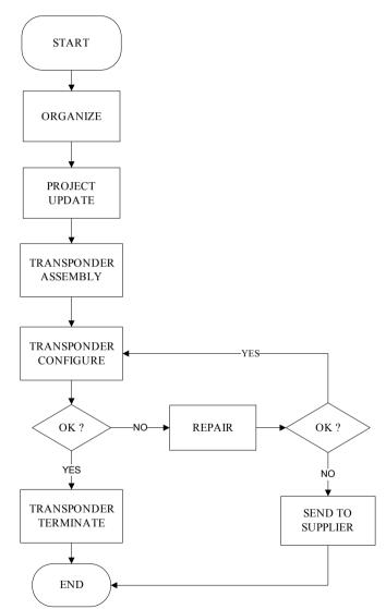
Figure 2 - Flow chart of the transponder A process, the simulation conceptual model
